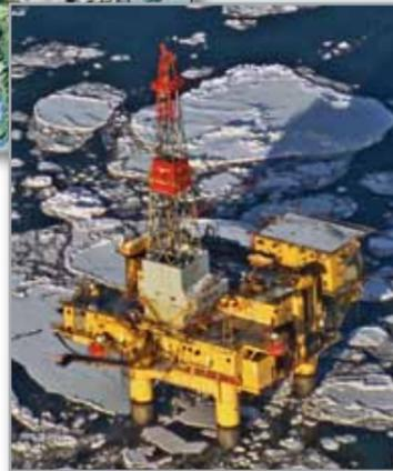
Top: Significant gas related activity occurs in Cook Inlet. Oil rigs must be able to withstand strong tidal currents and large chunks of sea ice. (AlaskaStock)
